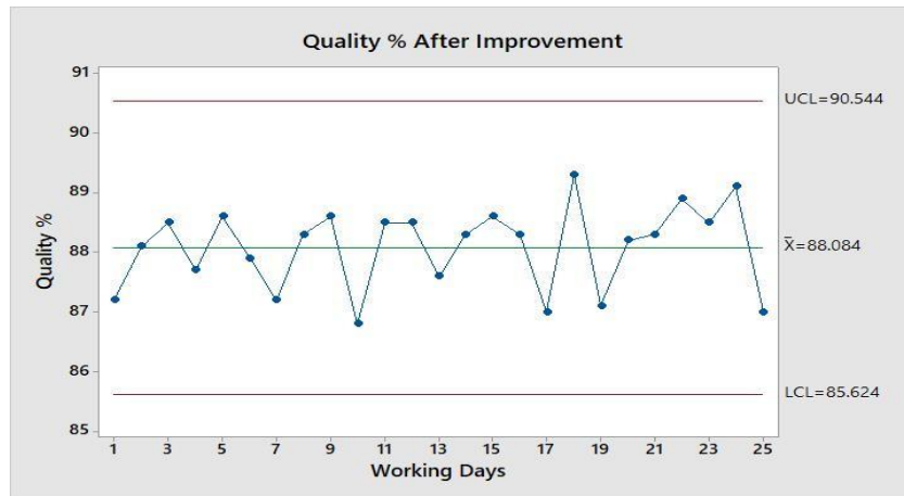
Fig. 15. Quality control chart (after improvement).
