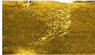
Figure 19 Side scan sonar and echo sounder data extracts showing seafloor sediments distribution
