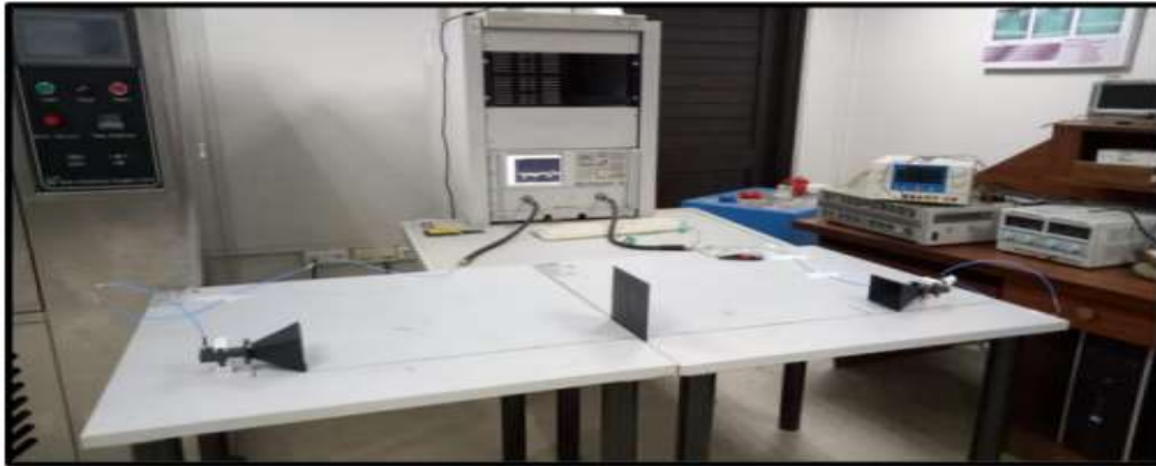
Fig. 6. Measuring shielding effectiveness using agilent e8362b PNA series
