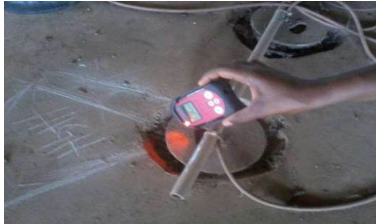
Fig. 6. Gamma survey meter recording value at “high point” of roof plug 3
