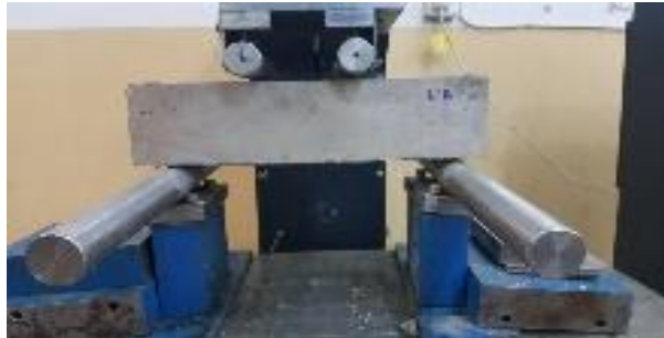
Fig. 2. Concrete beam under testing for flexural strength
