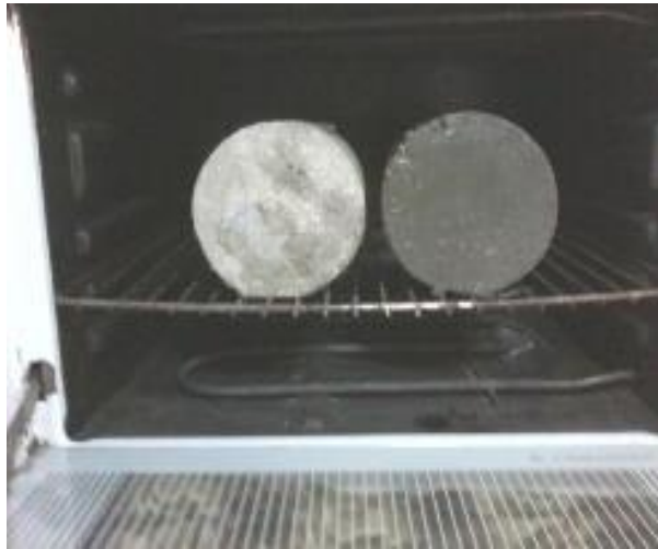
Fig. 3. Drying specimens in the oven for absorption test
