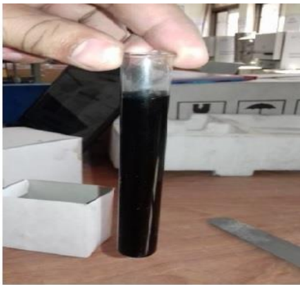
Fig. 2. CNTs after dispersion
