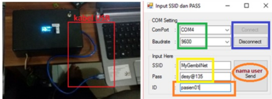
Fig. 9 . Setting SSID to the device
