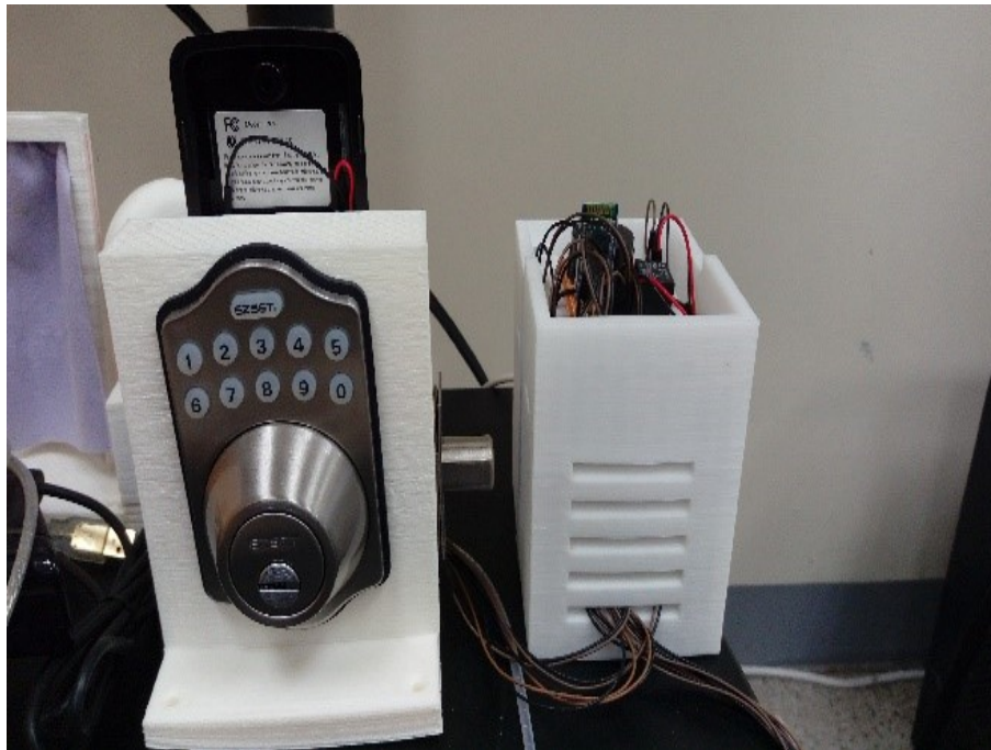
Fig. 6. Entrance guard system and Arduino microcontroller system
