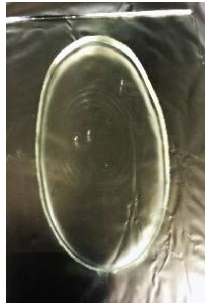
Fig. 3. The spiral microchannel following its manufacturing in PDMS.
