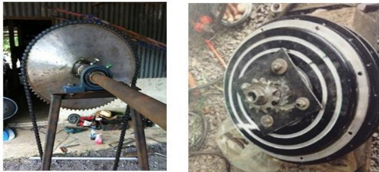
Fig. 11 . Gear of turbine axis and gear of electric bicycle motor
