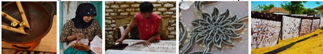
FIGURE 4 Canting of the Batik Tulis, Batik Drawing Activity (batik Tulis & Cap) and the Processed Product
