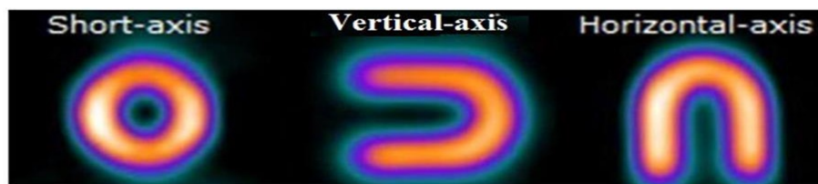
Fig. 4 . Non-uniformity of SPECT image in 3 views; short-axis, vertical-axis, and horizontal-axis
