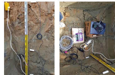
Fig. 4. Measuring the electrical properties of clayey sand
