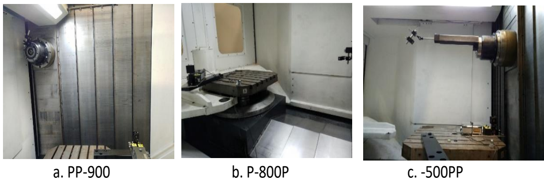
Fig. 4. Set-ups of measurement of face diagonal of each plane
