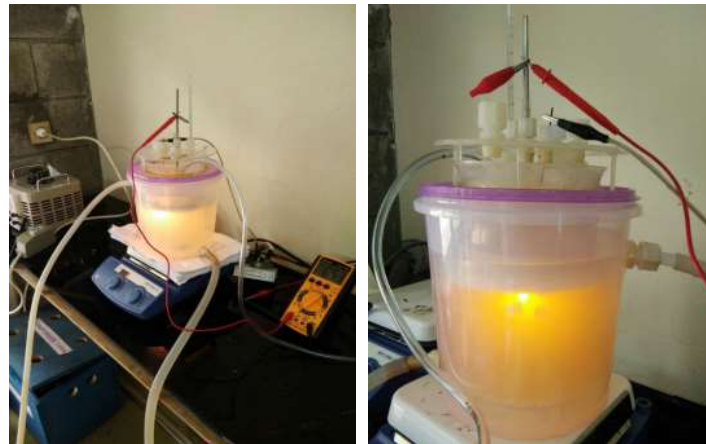
Fig. 5. (a) The experimental setup of the plasma electrolysis (b) Plasma that occurred in the reactor
