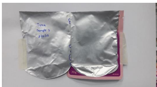
Fig. 12. Laminated film with 2.5 kW. corona treated on aluminum surface that held tuna paste for 30 days
