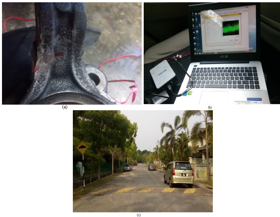
Fig. 4. Capturing the fatigue strain signal process: (a) Strain gauge mounted on the steering knuckle, (b) Data acquisition system, (c) Condition of the road surface
