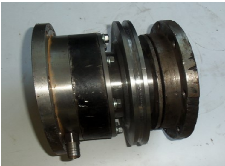
Fig. 7 . Photo of the prototype of the hydro turbine 20 cm in length
