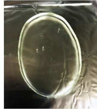
Fig. 3. The spiral microchannel following its manufacturing in PDMS.
