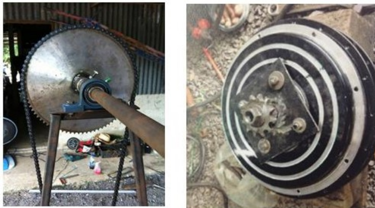
Fig. 11 . Gear of turbine axis and gear of electric bicycle motor
