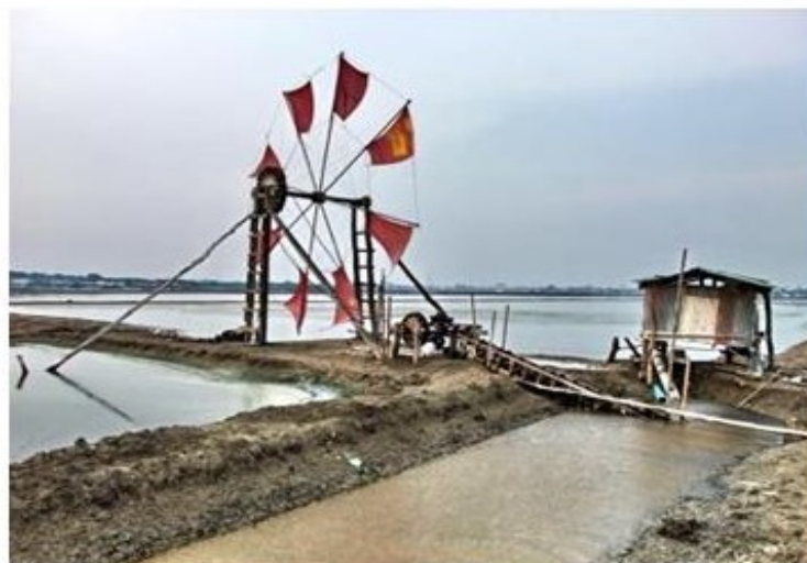
Fig. 4 . Saline wind turbine at Thai gulf coastline [11]
